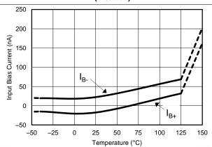
Figure 9. Input Bias Current vs Temperature (Enabled)
