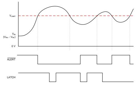
Figure 29. Transparent versus Latch Mode
