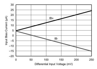
Figure 31. Input Bias Current vs Differential Input Voltage
