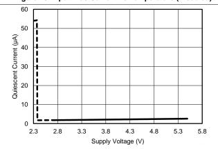
Figure 11. Quiescent Current vs Supply Voltage (Enabled)
