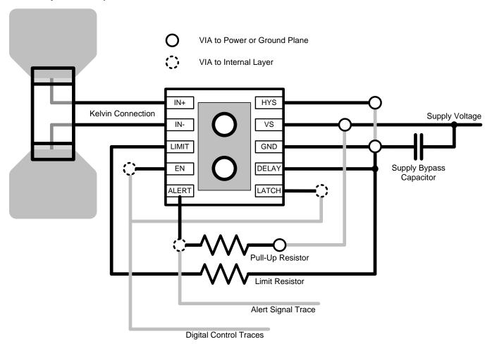
NOTE: Connect the limit resistor directly to the GND terminal.
