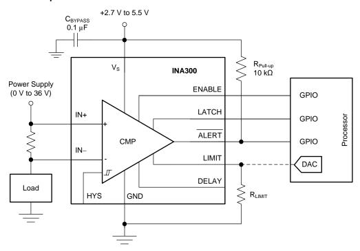
Figure 33. Unidirectional Application Schematic
