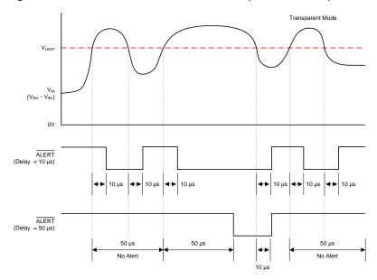
Figure 22. DELAY Terminal Settings
