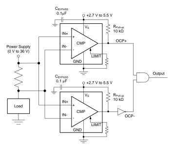
Figure 37. Window Comparator Application
