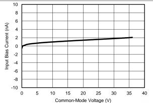
Figure 7. Input Bias Current vs Common-Mode Voltage (Enabled)
